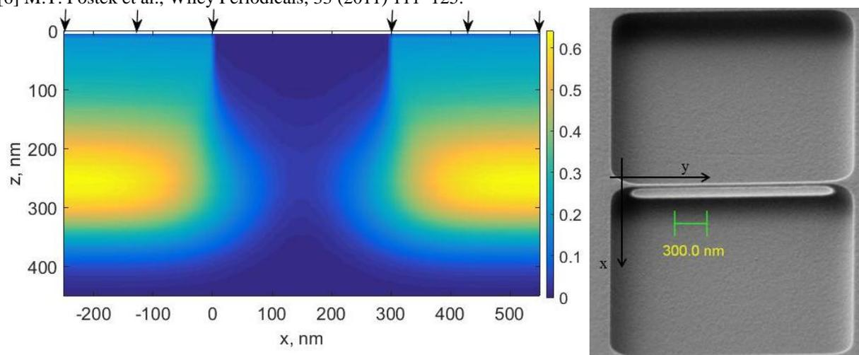
Figure 1. (a) Map of calculated ion-induced defects concentration, there is a slight overlapping between the irradiated areas (arrows on the top show the ion beam); (b) 45-deg tilt SEM images of neighboring areas after under etching through the wall of the volume with overlapping of defects.
