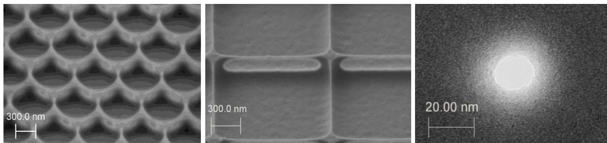
Figure 1. Images of examples of the nanostructures fabricated by means of ion beam enhanced etching. (a) SEM image of honeycomb type structure; (b) SEM image of suspended nanostrings; (c) TEM image of single nanopore in silicon nitride
